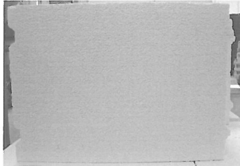
Fig. 5. Rough surface of cement and sulphate free AAC
