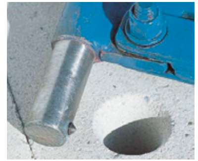
B. Approved clamping device for lifting the Silka elements with a element stacker.
