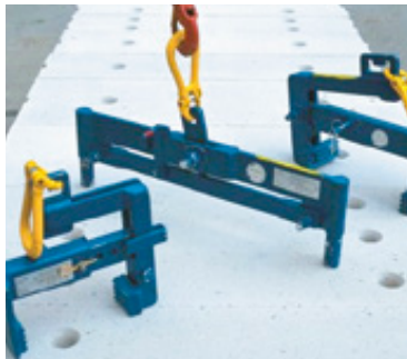
C. Clamping devices for lifting cut blocks with the element stacker.
