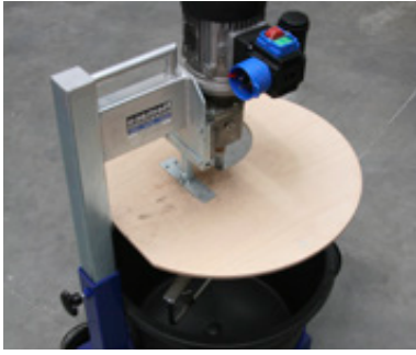
I. Plastic mortar trough for mixing the thin joint mortar.
