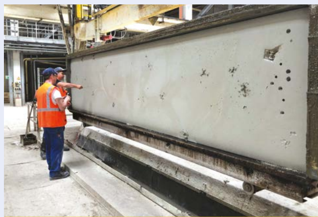
Production of 5.4 m 3 AAC (Ytong PP2-0,35) with LT-BCC in the large-scale pilot plant of Xella Technology and Research. Here, 25% of the ordinary portland cement (OPC) was substituted with LT-BCC.
